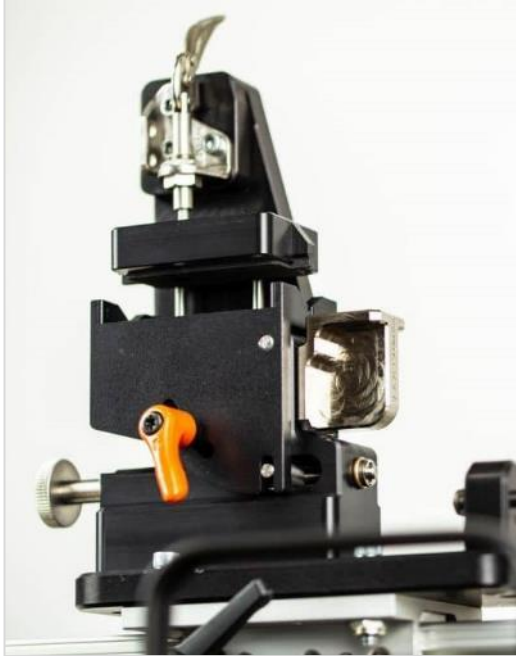
CATHETER TIP DEFLECTION FIXTURE
