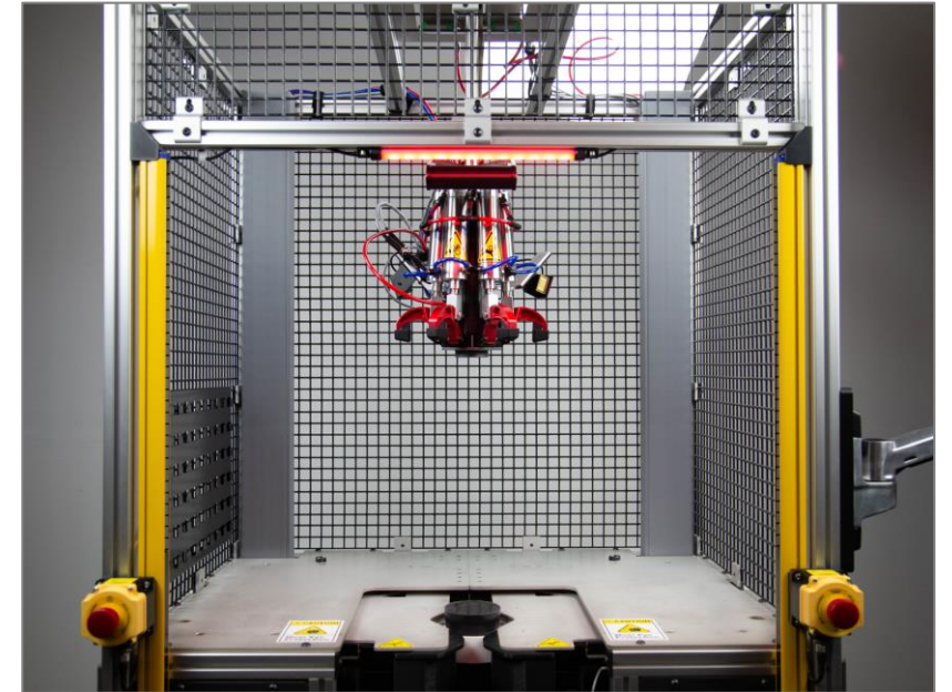
AUTOMATED DEMOLDING CELL
